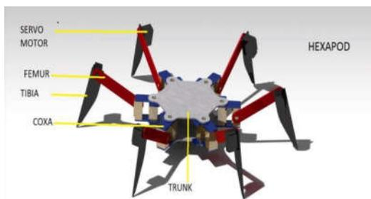
Figure: 3D model designed in CATIA
