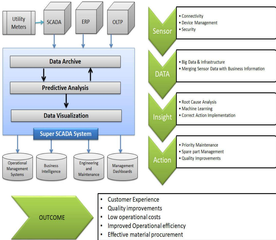
Figure-6.1: Proposed Super SCADA System applications and outcome
