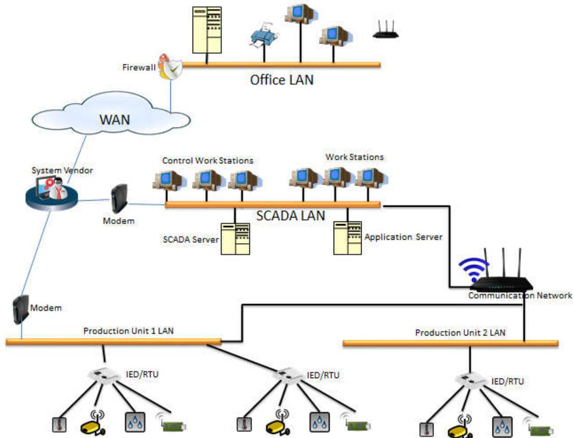
Figure- 3.4: Fourth Generation SCADA Systems (Currently Used)
