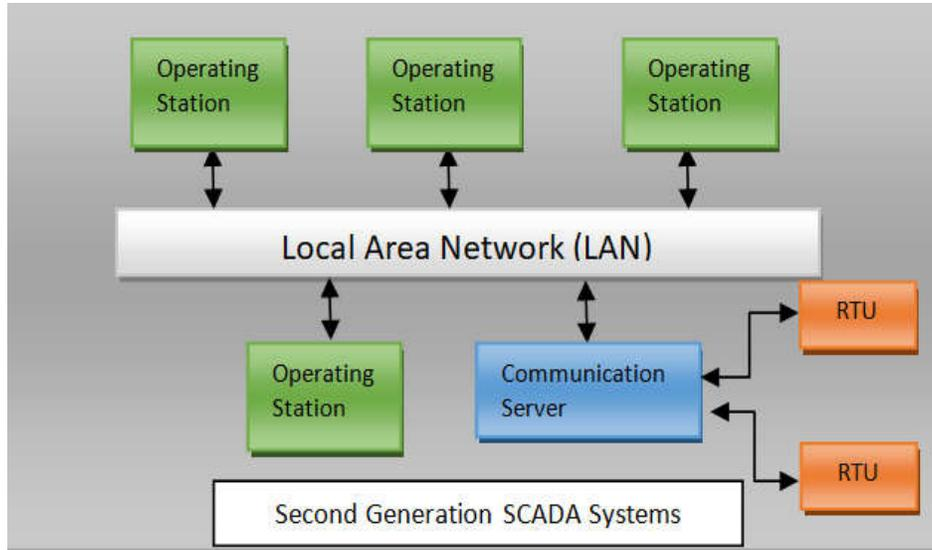
Figure-3.2: Second Generation SCADA Systems
