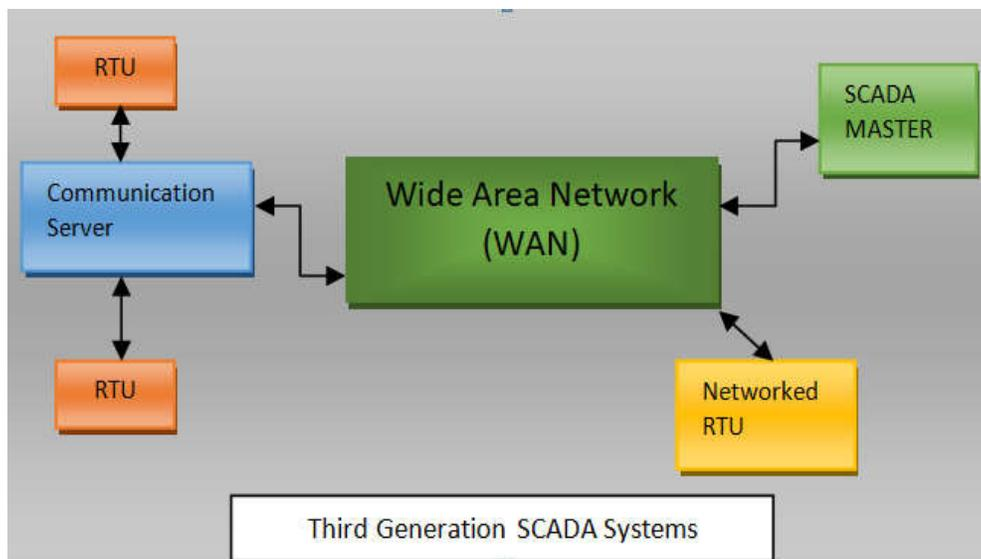
Figure-3.3: Third Generation SCADA Systems
