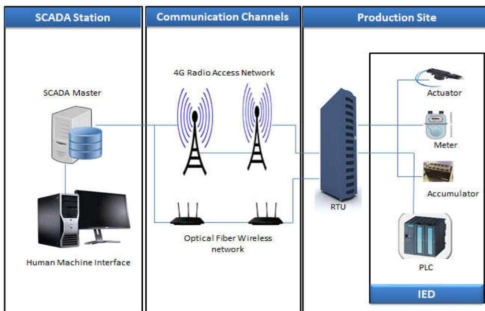
Figure-2.1: SCADA Components
