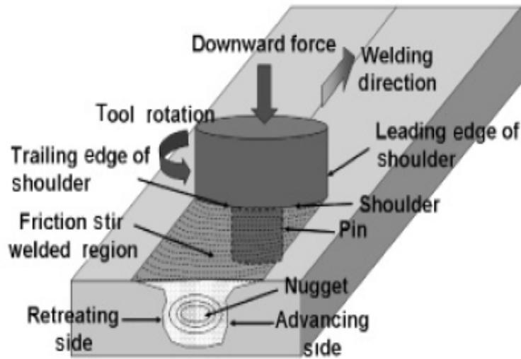
Figure 1. Schematic representation of FSW technique [6]
