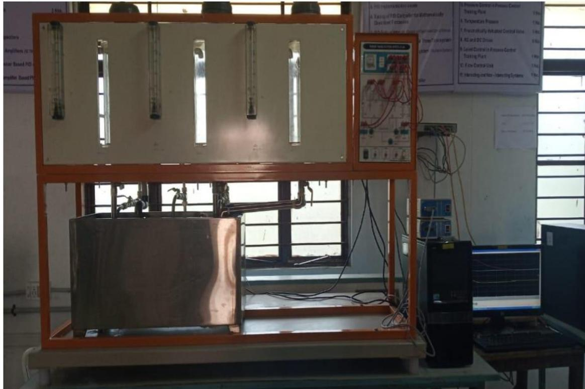
Fig.8 Experimental setup of three tank interacting system
