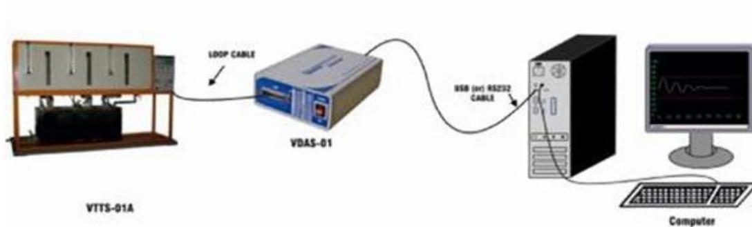
Fig. 4 Interfacing Diagram Of Three Tank System
