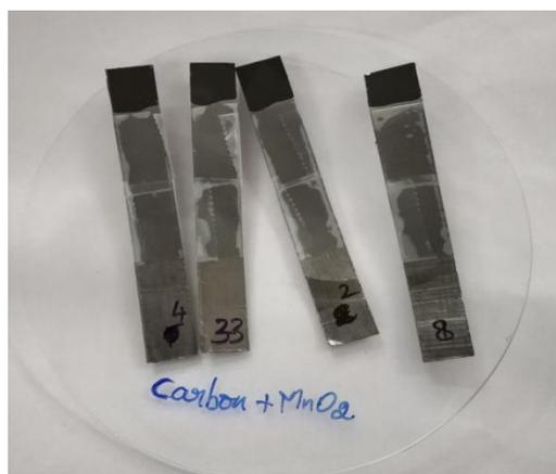
Figure 5. Shows  $\text{MnO}_2$  coated carbon electrode
