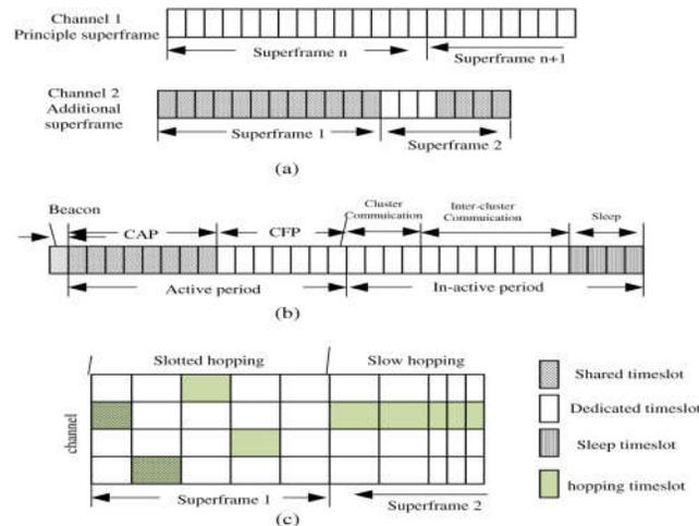
Fig. 3. Super frame structure of the mainstream IWSN standards: (a) Wireless HART (b) WIA-PA (c) ISA100.11a
