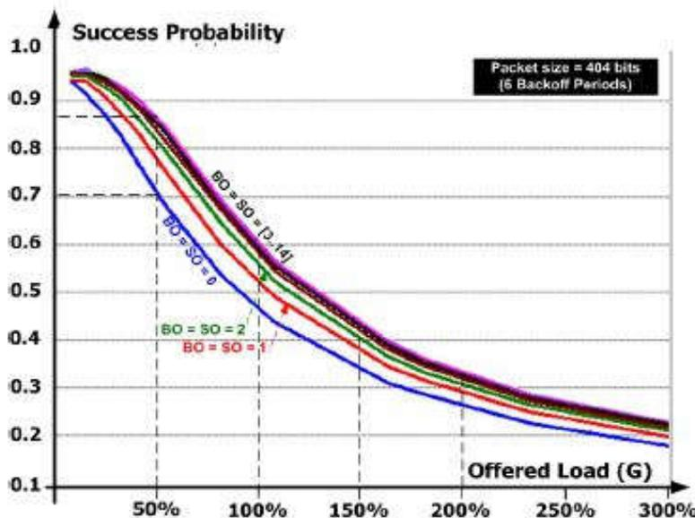
Fig. 5. Success probability as a function of the offered Load for different (BO, SO) values
