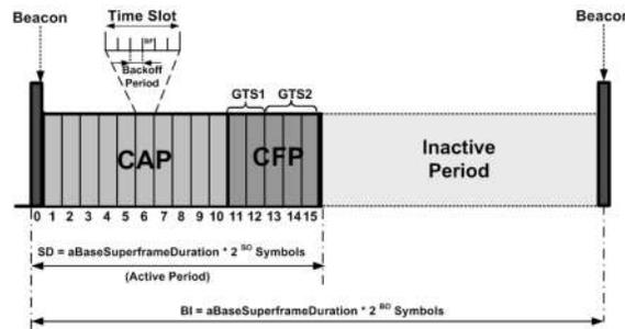
Fig. 2 Super frame structure of IEEE 802.15.4
