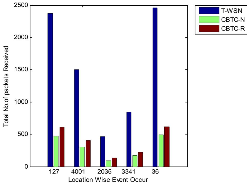
**Comparison of T-WSN and CBTC with respect to numbers of packets received.**
