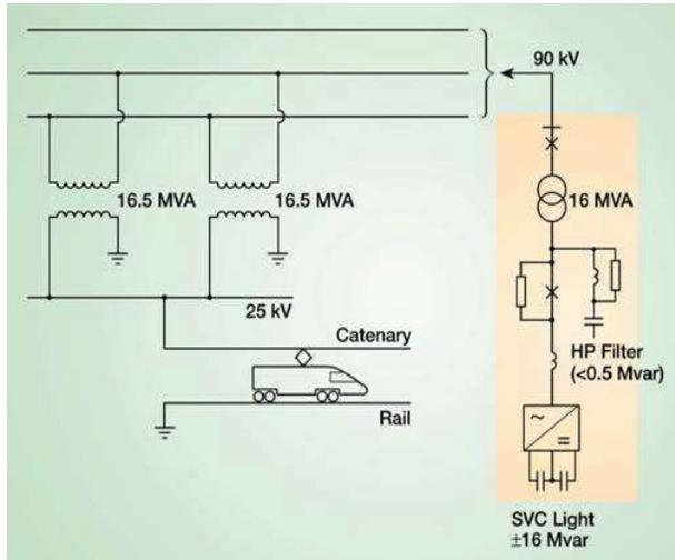
Fig -: 6 SVC Light for 90 kV, 16 MVA.
