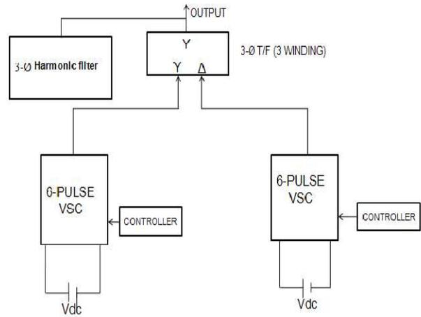
Figure-: 5 Block diagram of 12-pulse voltage source converter STA TCOM with harmonic
