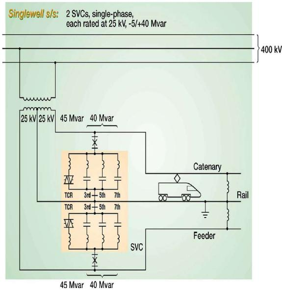
Fig -: 4 application of 2 SVC in traction system
