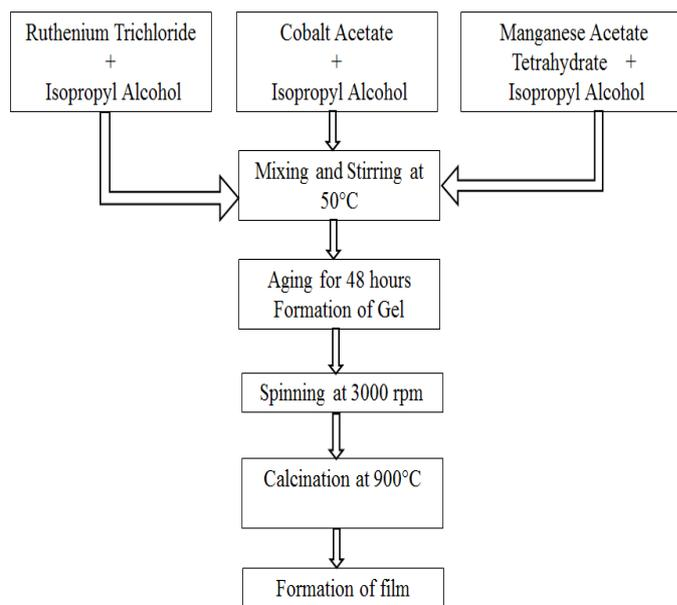
Fig. 1. Flow chart for deposition of [Co:Mn:Ru] Oxide Composite Thin Film
