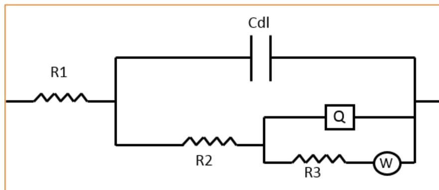
Fig. 9. A equivalent circuit for [Co:Mn:Ru] Oxide composite thin films electrodes
