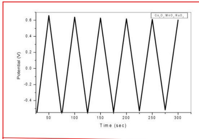
Fig.6. Charge-discharge curves of composite [Co:Mn:Ru] oxide thin film electrode
