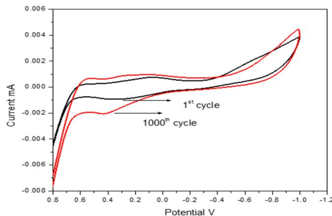
Fig. 7. Cyclic stability composite [CO:Mn:Ru] oxide thin film electrode
