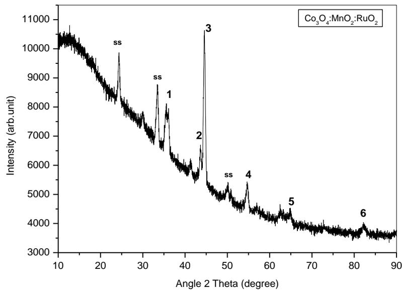
Fig. 2. XRD patterns of [Co:Mn:Ru] oxide thin film
