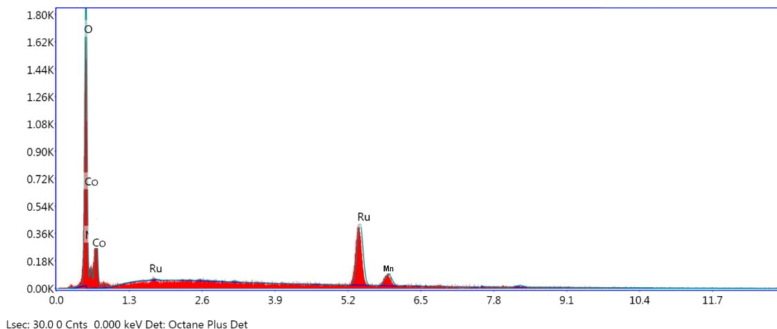
Fig. 4. EDAX patterns of [Co:Mn:Ru] oxide thin film
