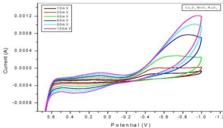
Fig. 5. Cyclic Voltammograms of ternary composite [Co:Mn:Ru] oxide thin film electrode
