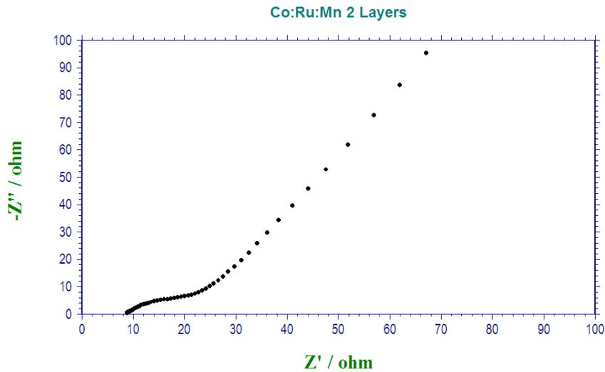
Fig. 8. Impedance Spectroscopy (Nyquist Plot) composite [CO:Mn:Ru] oxide thin films electrodes
