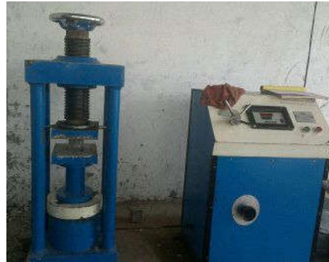
Figure: 1 Compressive Strength Testing of Cubes Samples
