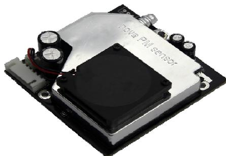
Figure 5. Nova PM sensor SDS011 [9]
