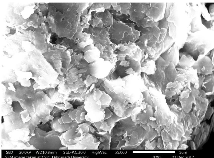
**Fig9:** SEM photograph of sample having depth 3076.54m shows the presence of kaolinite and illite with platey nature
