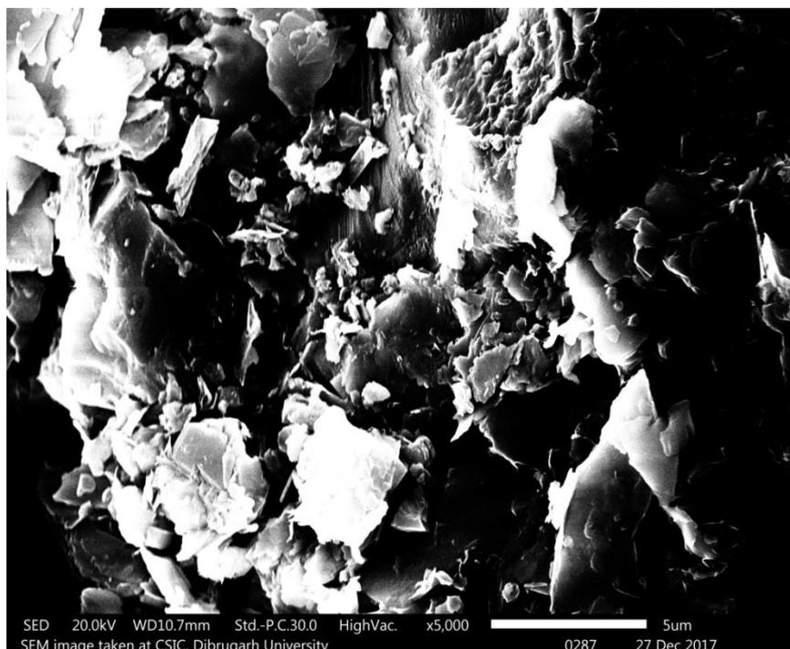
**Fig8:** SEM photograph reveals the presence of smectite with honeycomb nature of sample having depth 2707.50m
