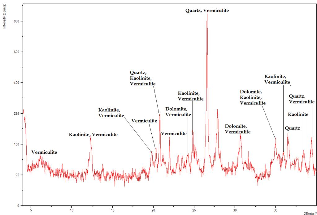
**Fig6:** XRD of sample having depth 3076.36m
