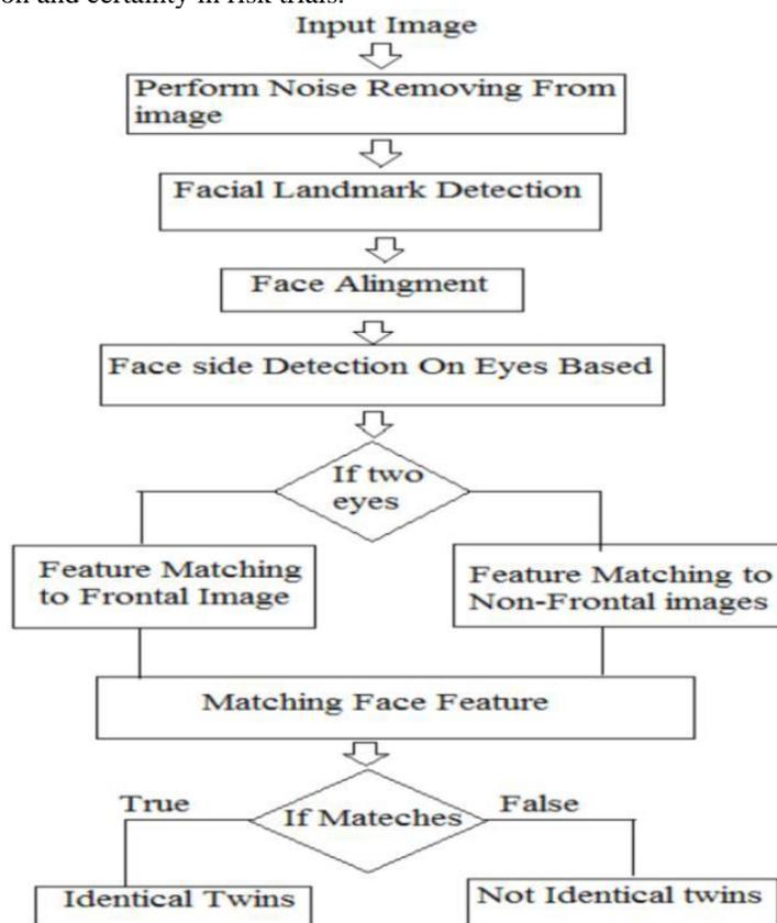
**Figure 1:** Process flow of Detection of Identical twins
