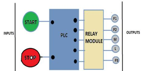
Figure 11. Wiring of components with PLC kit
