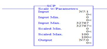
Figure 9. Scale with Parameter
