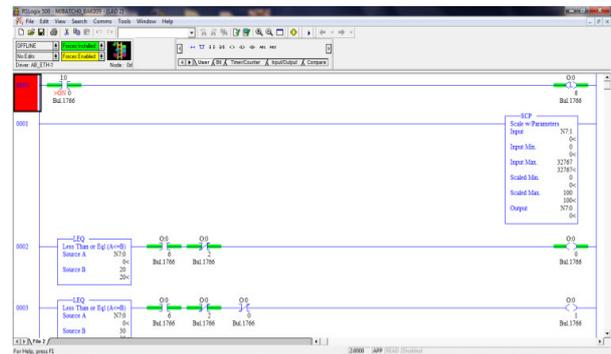
Figure 12. Logic to Maintain the Ratio
